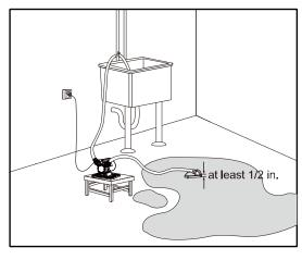
6. To operate, plug the cord into a 3-wire, 115V, 60Hz, grounded GFCI outlet.
