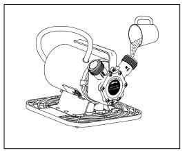
1. Fill water into inlet and outlet of the pump to wet the impeller.
