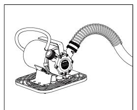
3. Thread the other end of the suction hose onto the suction inlet of the pump
