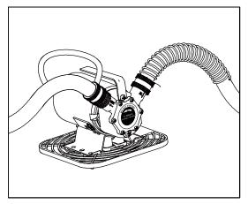
4. Thread a 1/2in. or larger garden hose (sold separately, 50 ft max. length) onto the discharge outlet of the pump.
