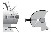
Brush must enter square hole. → Match brush curve to armature curve
