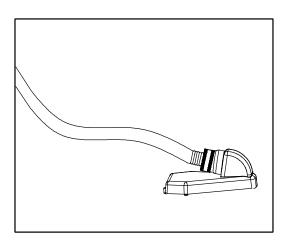
2. Attach suction hose by pushing the male threaded end into the rubber suction strainer, then place the strainer in at least 1/2 in. of water at the lowest point to be pumped. **NOTICE**: Make sure the connection is airtight. An air leak can cause the pump to run dry.
