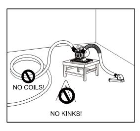
5. Secure the pump solidly on a stable platform (table, board, etc.) to prevent it from tipping over. Make sure the hoses are as straight as possible.
