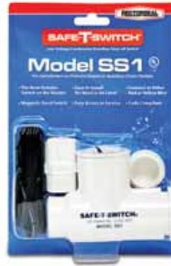
**Application** • Detects clogged A/C condensate drains and shuts off the system to prevent water damage to floors, walls and ceilings • Can be installed horizontally or vertically, inline or on the primary pan's auxiliary drain outlet by using the included 3/4" adapter, bushing and cap • Can be installed on a sloping line and does not need to be level or plumb
