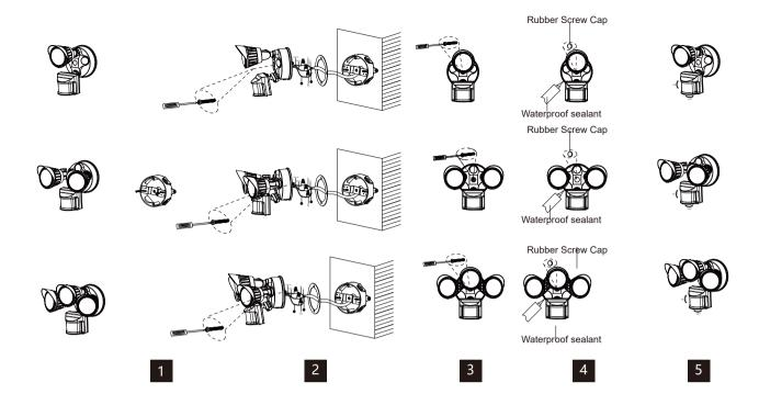
1. Fixing the bracket installation hole with junction box hole by screw, the screw included in accessory bag.
