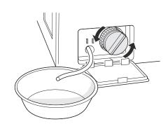
Clean the pump filter and opening.
