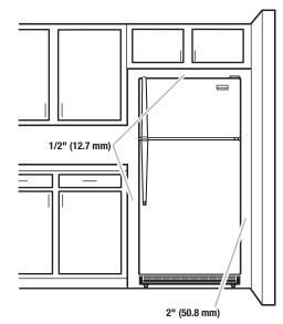
To ensure proper ventilation for your refrigerator, it is recommended to allow a 1/2" (1.27 cm) space on each side and between overhead cabinets and refrigerator top. Allow at least 1" (2.54 cm) between back of cabinet and the wall. If your refrigerator has an ice maker, make sure you leave extra space at the back for the water line connections.
