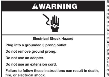
**Electrical:** A 115 V, 60 Hz, AC only, 15 A or 20 A fused, grounded electrical supply is required. It is recommended that a separate circuit serving only your refrigerator be provided. Use an outlet that cannot be turned off by a switch. Do not use an extension cord.
