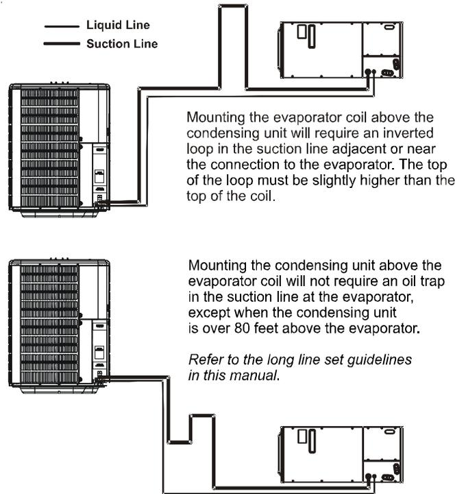
Insulation is necessary to prevent condensation from forming and dripping from the suction line. Armflex (or satisfactory equivalent) with 3/8" min. wall thickness is recommended. In severe conditions (hot, high humidity areas) 1/2" insulation may be required. Insulation must be installed in a manner which protects tubing from damage and contamination.
